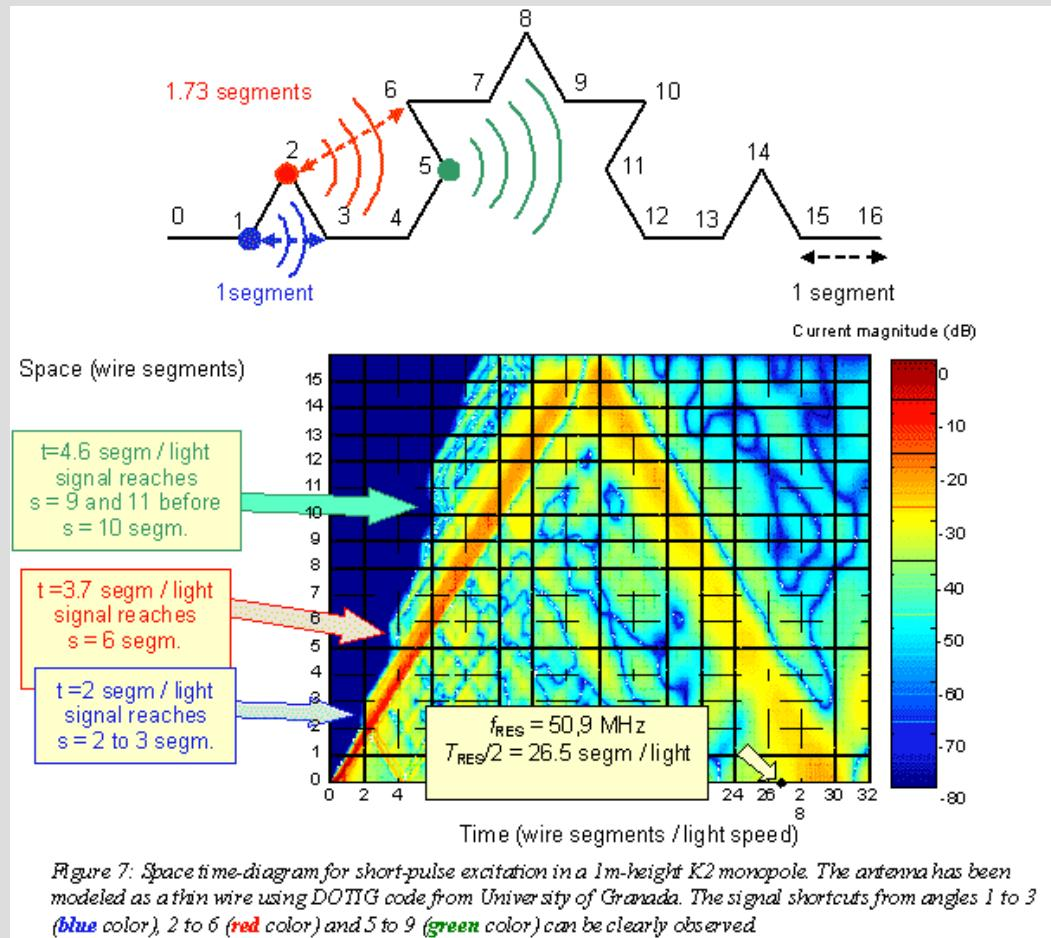
Figure 7: Space time-diagram for short-pulse excitation in a 1m-height K2 monopole. The antenna has been modeled as a thin wire using DOTIG code from University of Granada. The signal shortcuts from angles 1 to 3 (blue color), 2 to 6 (red color) and 5 to 9 (green color) can be clearly observed
